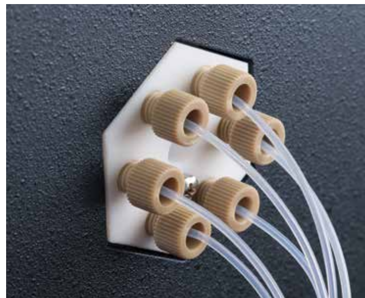
Autosampler Stream Selection Valve
